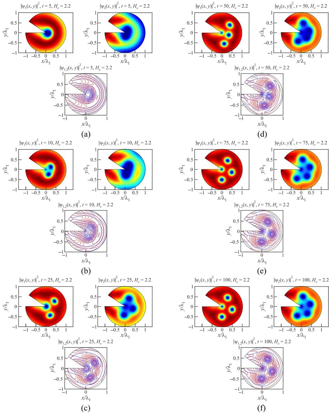
Fig. 4. Time evolution of magnetic flux penetration inside the two-band superconductor specimen with a cross-section in form of the circle with a triangular cutout, settled in external magnetic field ( $H_e = 2.2$ ) at different time moments after the turning on the magnetic field,  $t$ : 5 (a), 10 (b), 25 (c), 50 (d), 75 (e), 100 (f).
