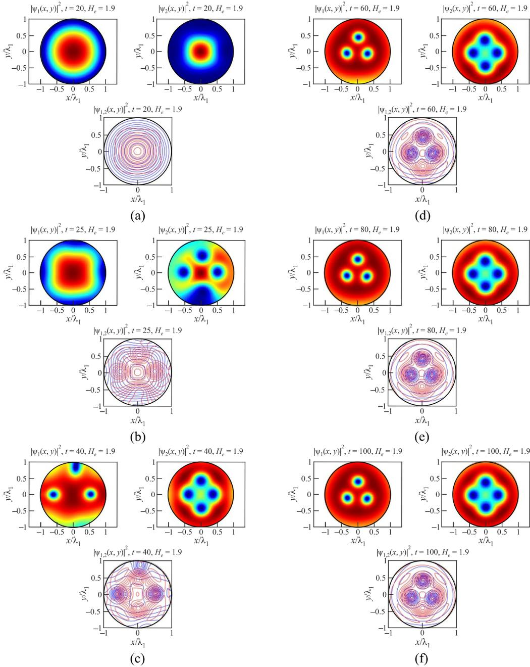
Fig. 3. Time evolution of magnetic flux penetration inside the circular two-band superconductor settled in external magnetic field ( $H_e = 1.9$ ) at different time moments after the turning on the magnetic field,  $t$ : 20 (a), 25 (b), 40 (c), 60 (d), 80 (e), 100 (f).
