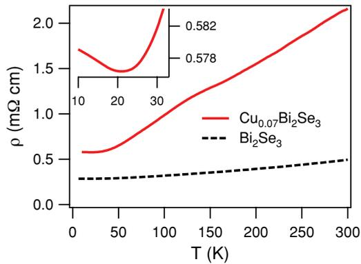
FIG. 1. (Color online) In-plane resistivity of the pure (black dashed line) and Cu intercalated (red solid line)  $\text{Bi}_2\text{Se}_3$  crystals; the low-temperature region of the later is zoomed in the inset.
