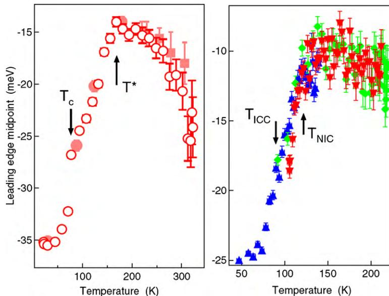
**Fig. 4.** Non-monotonic gap function. The position of the leading edge midpoint (LEM) of the integrated  $k_F$  EDCs (averaged for two Fermi-crossings), as function of temperature for an underdoped Tb-BSCCO (left) [12] with  $T_c = 77$  K and  $T^* = 170$  K is remarkably similar to the pseudogap in a transition-metal dichalcogenide TaSe<sub>2</sub> (right) [13] with the transitions to the commensurate and incommensurate CDW phases at  $T_{ICC} = 90$  K and  $T_{NIC} = 122$  K, respectively.
