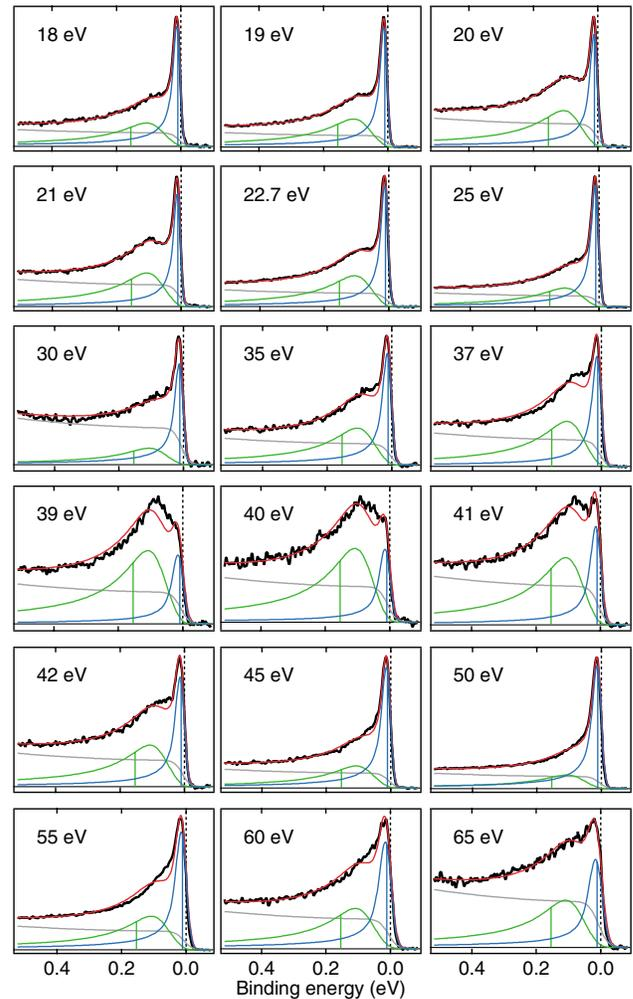
FIG. 2 (color). The  $(\pi, 0)$  photoemission spectra from the superconducting state of an overdoped (69 K) sample for different excitation energies: the black lines show the experimental data and the colored lines represent the results of a fitting procedure described in the text.
