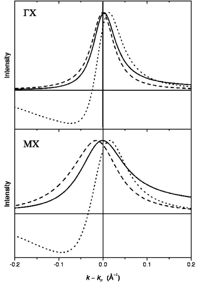
FIG. 6. Results of  $E_F$ -MDC simulations for nodal [ $\Gamma$ - $(\pi, \pi)$  crossing, upper panel] and antinodal [ $(\pi, 0)$ - $(\pi, \pi)$  crossing, lower panel] ARPES data for a typical low-energy dispersion (for details see text). The dashed curves are the raw (non-normalized) MDC’s, the solid curves are the MDC’s after self-normalization to the highest binding energy, and the dotted curves represent the results of the  $dn(k)/dk$  method.
