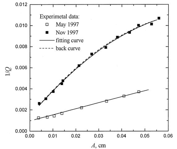
Fig. 1. The experimental dependencies of the inversed  $Q$ -factor on the resonance amplitude of the permanent magnet above the bulk YBCO sample just after manufacturing ( $\square$ ) and in half a year ( $\blacksquare$ ); the dashed curve ('back' curve) represents the dependence obtained back from Eqs. (1), (5), (10) and (12).
