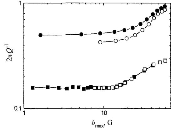
**Fig. 1.** The reverse  $Q$ -factor vs the maximum amplitude of magnetic field on the HTSC surface for the ceramic (closed symbols) and composite (open symbols) samples made of  $\text{YBa}_2\text{Cu}_3\text{O}_{7-x}$  (squares) and  $(\text{Pb}_{0.16}\text{Bi}_{0.84})_2\text{Sr}_2\text{Ca}_2\text{Cu}_3\text{O}_y$  (circles) superconductors.
