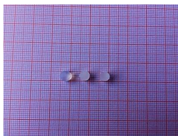
Fig. 8. Photograph of \text{SiO}_2\text{CeAr} xerogel of silica after irradiation with different gamma ray doses.
