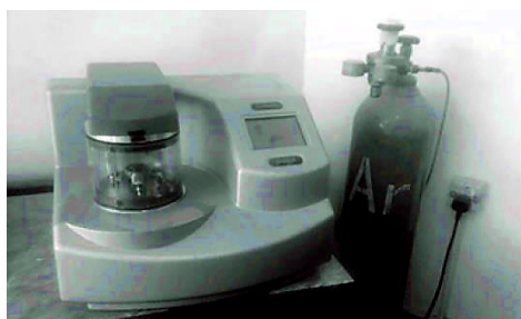
Fig. 2. Q150R ES device used to deposit nanogold layer.
