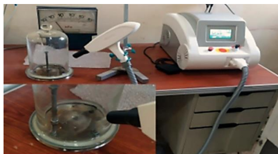
Fig. 2. The Nd:YAG pulsed laser instrument.
