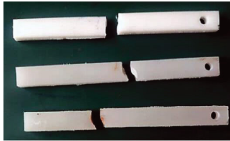
Fig. 6. Samples from fatigue tests following failure.
