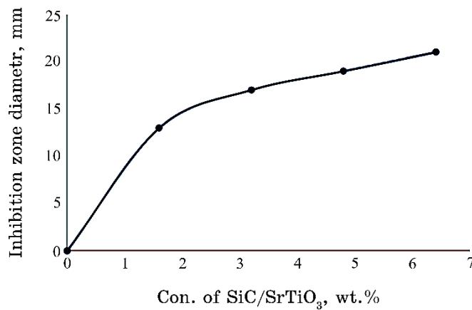
**Fig. 3.** Inhibition zone diameter of PMMA/PEO/SiC/SrTiO<sub>3</sub> nanostructures against *Staphylococcus* bacterium.
