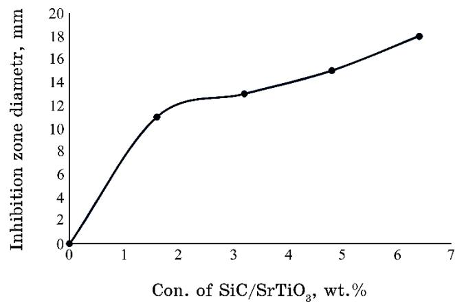
**Fig. 2.** Inhibition zone diameter of PMMA/PEO/SiC/SrTiO<sub>3</sub> nanostructures against *Escherichia coli*.
