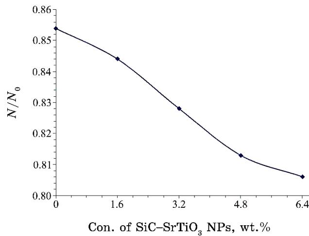
**Fig. 4.** Variance of ( $N/N_0$ ) for PMMA/PEO with different concentrations of SiC-SrTiO<sub>3</sub> NPs.
