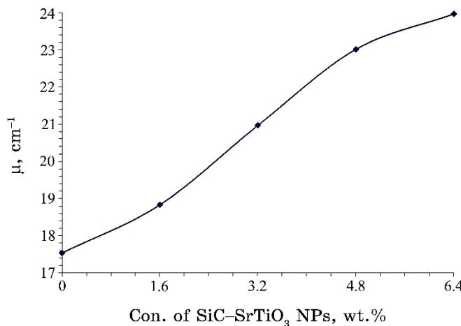
**Fig. 5.** Variance of attenuation coefficients of gamma-radiation for PMMA/PEO blends with different concentrations of SiC-SrTiO<sub>3</sub> NPs.
