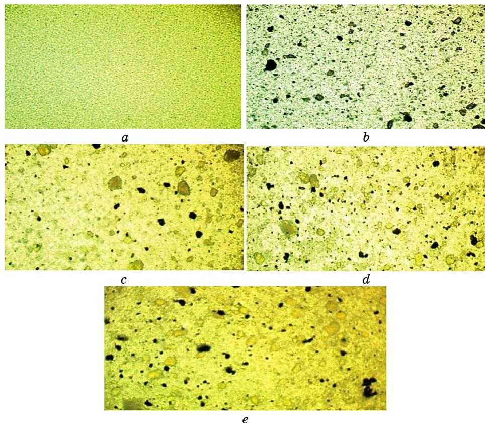
**Fig. 1.** Optical microscope images ( $\times 10$ ) for PMMA-PEO-SiC-SrTiO<sub>3</sub> nanostructures: (a) pure; (b) 1.6 wt.% SiC-SrTiO<sub>3</sub> NPs; (c) 3.2 wt.% SiC-SrTiO<sub>3</sub> NPs; (d) 4.8 wt.% SiC-SrTiO<sub>3</sub> NPs; (e) 6.4 wt.% SiC-SrTiO<sub>3</sub> NPs.
