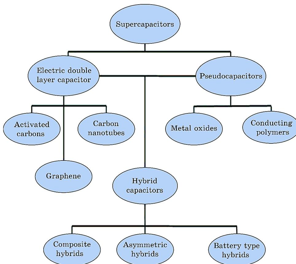
Fig. 2. Classification of supercapacitors (courtesy [3]).
