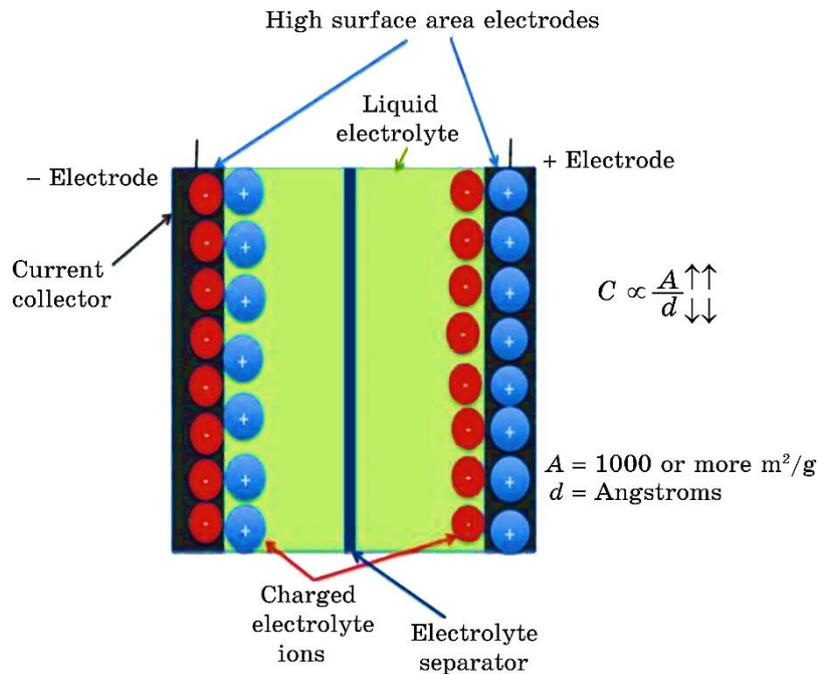
Fig. 1. Supercapacitor (courtesy [3]).
