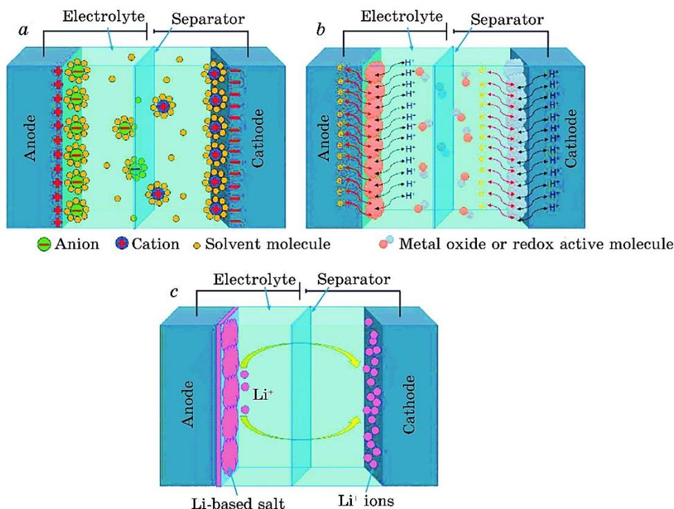
**Fig. 3.** (a) Electrical double layer capacitor (EDLC); (b) pseudo-capacitor (PC); (c) hybrid supercapacitor (HSC) (courtesy [5]).
