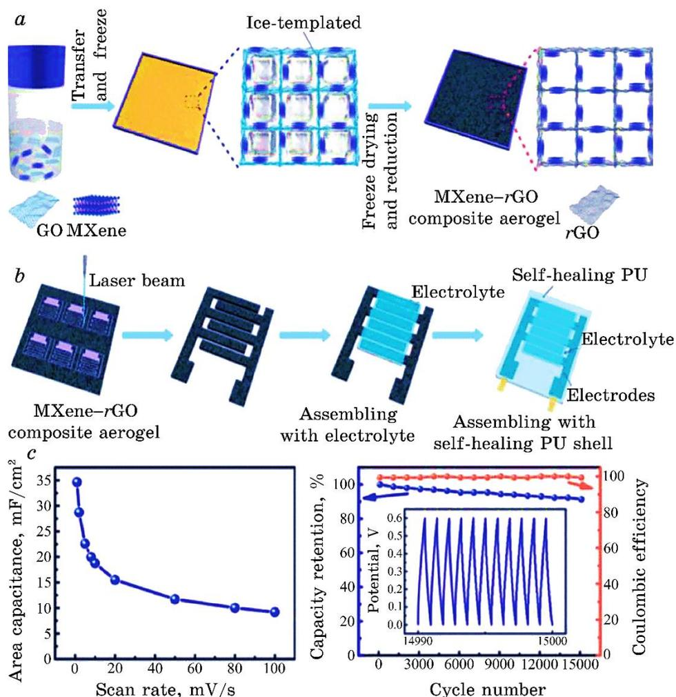
**Fig. 6.** (a) Fabrication of MXene-rGO composite aerogels; (b) laser cutting of interdigital pattern on MXene-rGO composite followed by assembling with self-healing PU; (c) plot showing the areal capacitance *vs* scan rate MXene-rGO composite; (d) cycling stability of MXene-rGO composite aerogel MSC at 2 mA·cm<sup>-2</sup>.
