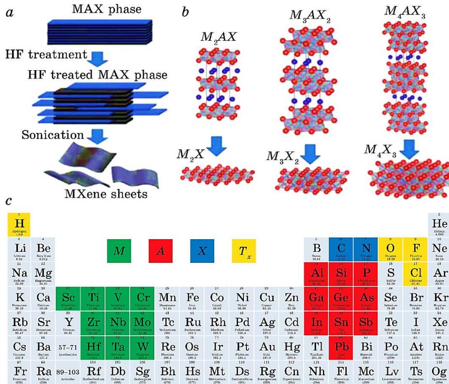
Fig. 4. (a) Schematic showing the synthesis of MXene from MAX by HF treatment; (b) synthesis mechanism of different order of MXenes by MAX phases; (c) compositions of MXene elements in periodic table (courtesy [31]).
