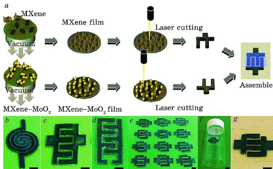
**Fig. 5.** (a) Fabrication process of MXene//MXene-MoO<sub>2</sub>-MSCs with different shapes such as spiral (b), parallel inter digital fingers (c, d), twelve parallel inter digital MSCs integrated on one paper (e), and MSCs transferred onto glass substrate (f) and cloth substrate (g) (courtesy [50]).
