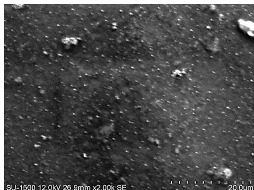
**Fig. 5.** SEM images of silver nanoparticles synthesized using stem extract of *O.indicum*.
