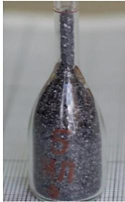
Fig. 1. Image of the powder of EG in the pycnometer.
