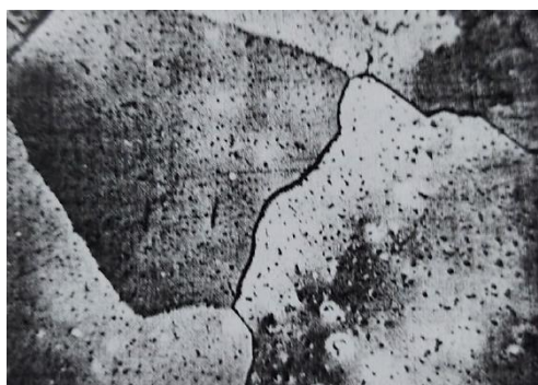
Fig. 1. Typical structure of disperse-reinforced material obtained from the vapour phase.
