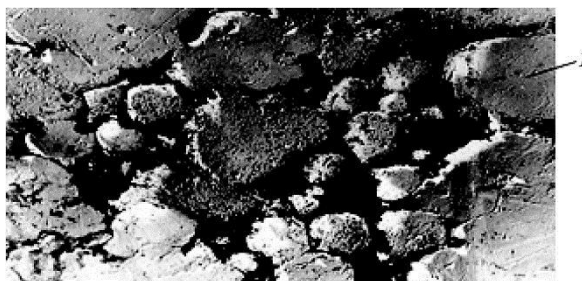
Fig. 9. The microstructure of an iron sponge was obtained by reducing the mill scale, \times 1000 . 1— \alpha -Fe.
