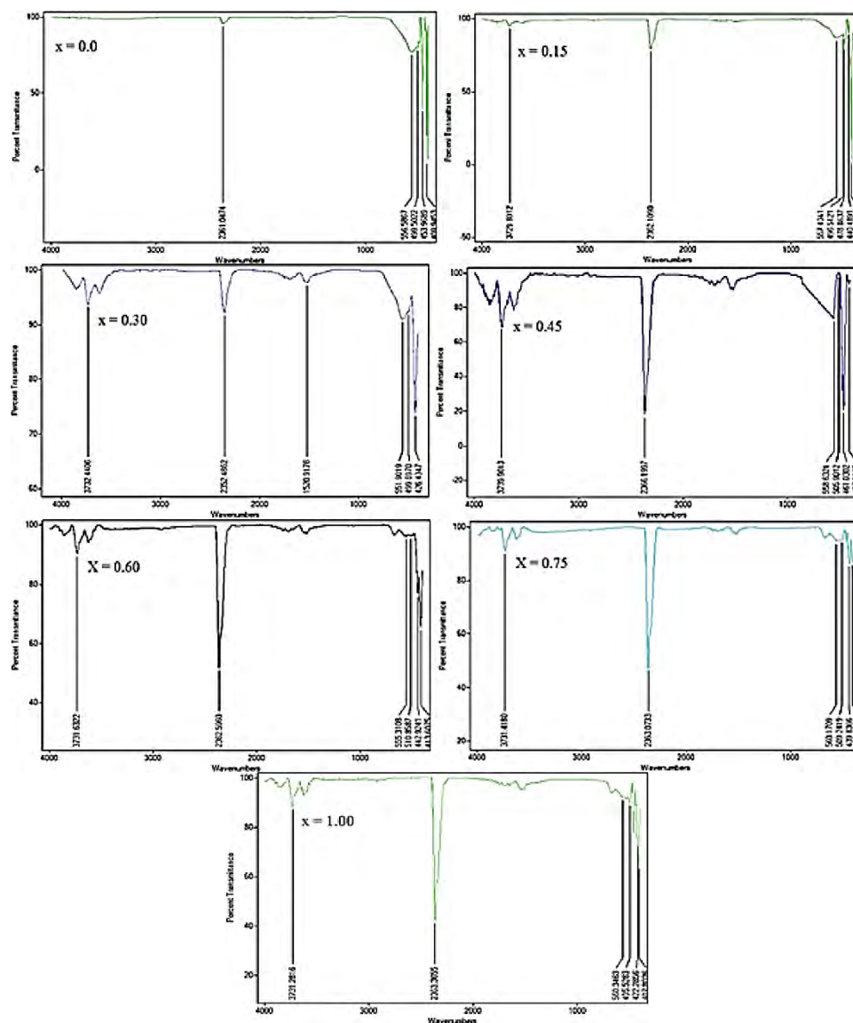
Fig. 3. FTIR spectrum of \text{Cu}_x\text{Mg}_{1-x}\text{NiFe}_2\text{O}_4 for x = 0.00, 0.15, 0.30, 0.45, 0.60, 0.75 , and 1.00 , respectively, synthesized at pH 7, calcined at 700^\circ\text{C} . They show octahedral and tetrahedral bonds between 400–600 \text{cm}^{-1} as characteristic of spinel ferrites nanoparticles.
