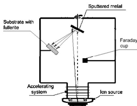
Fig. 1. Installation for metal-ion sputtering onto the fullerite.
