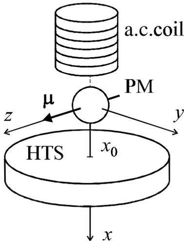
Fig. 3. Experimental configuration in resonance oscillations technique.
