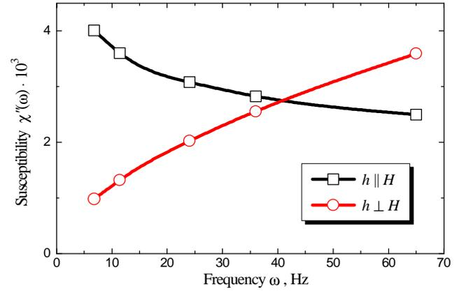
Fig. 4. Imaginary part of susceptibility vs alternating magnetic field frequency for longitudinal and transverse field components for Y-123 HTS.
