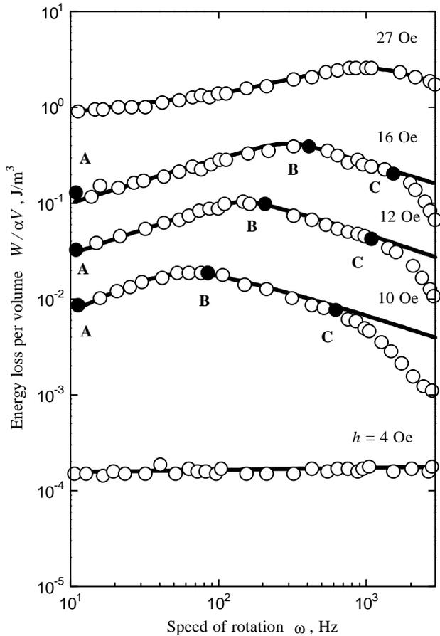
Fig. 5. Energy losses per volume of the HTS sample vs rotor's speed for the different field amplitude that depend on distance between HTS sample and rotor.
