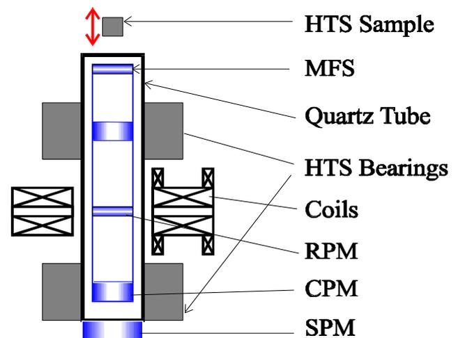
Fig. 2. Vertical configuration of rotor.
