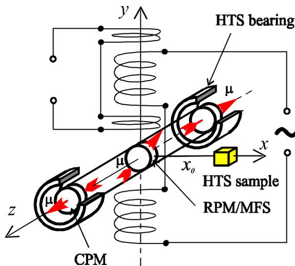
Fig. 1. Horizontal configuration of rotor for energy loss measuring.
